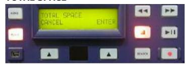
To verify the total capacity of your *DV Bank*, press the **MENU** button until TOTAL SPACE appears in the upper left corner of the LCD. Then press the Soft Key under the word **ENTER** and the total space available, as if there were no DV files stored on your *DV Bank*, will appear in the upper right corner of the LCD. Press the Soft Key under CANCEL to return to the FILE screen.
